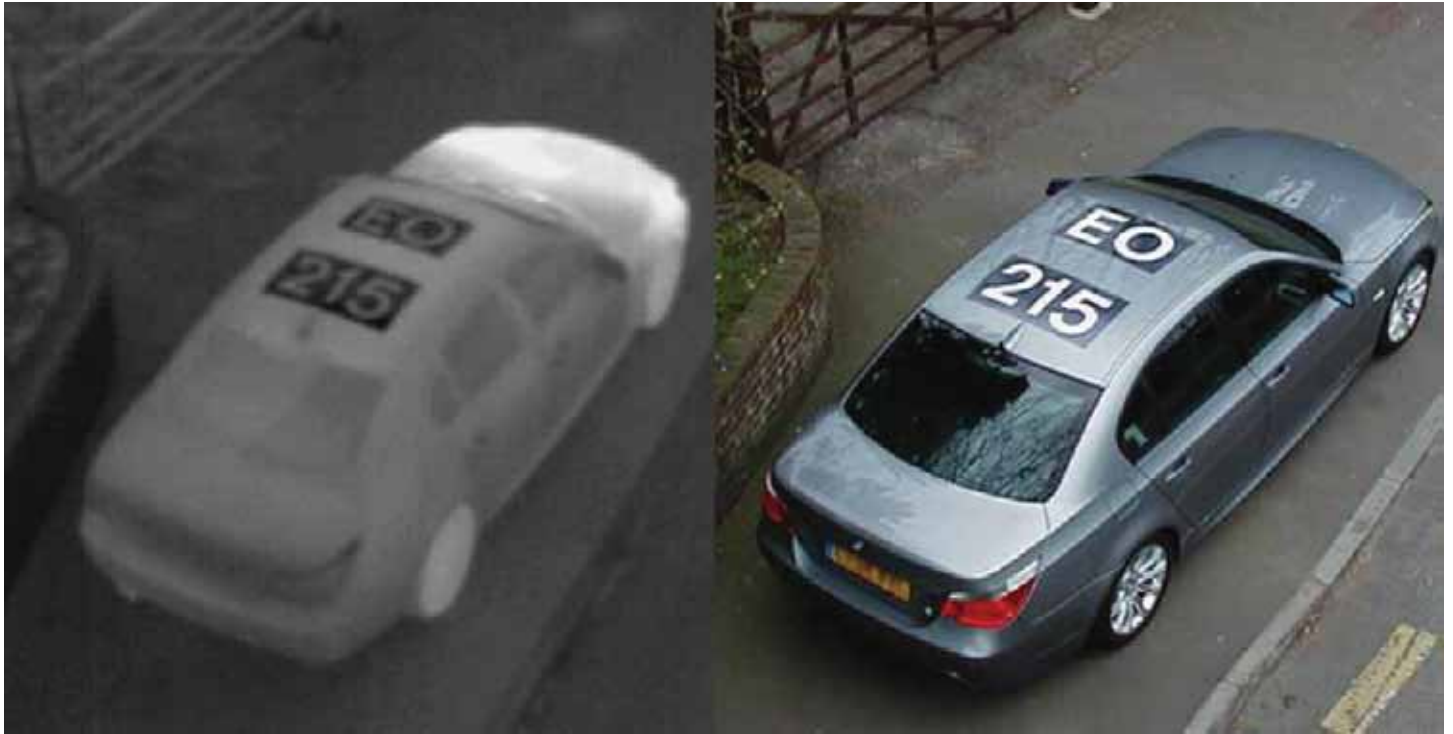
The images above show an unmarked test vehicle with Mirage H roof markings.
