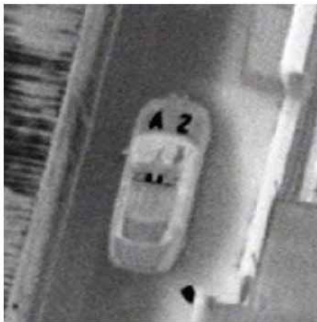
The above images show a police vehicle fitted with both Mirage™ and conventional roof markings. Only the Mirage™ markings are visible in the thermal infrared image.
