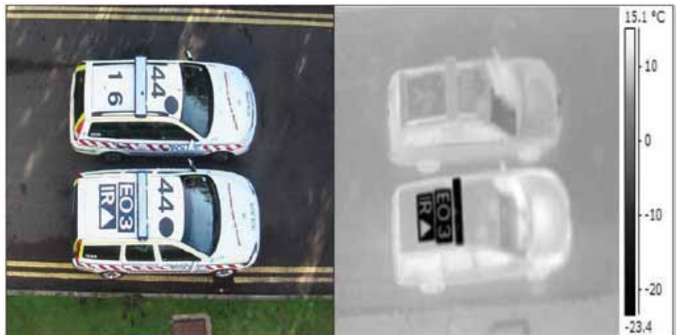
The images above show an unmarked test vehicle with Mirage H roof markings.
