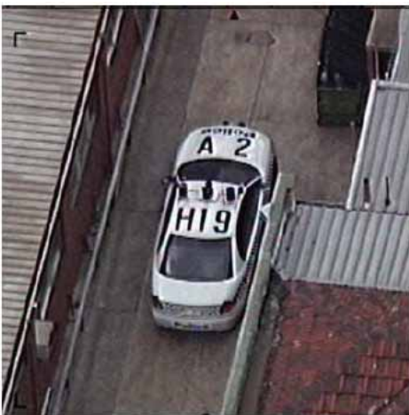
The above images show a police vehicle fitted with both Mirage™ and conventional roof markings. Only the Mirage™ markings are visible in the thermal infrared image.
